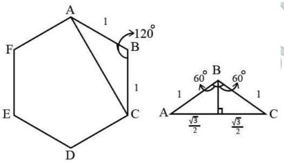
The length of the diagonals of a regular hexagon with side s are  $\sqrt{3}s$ .
